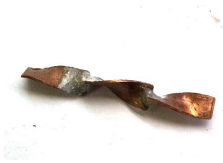
Figure 15 Flow mixer used at the exit of the microchannel to allow for more accurate temperature measurements
